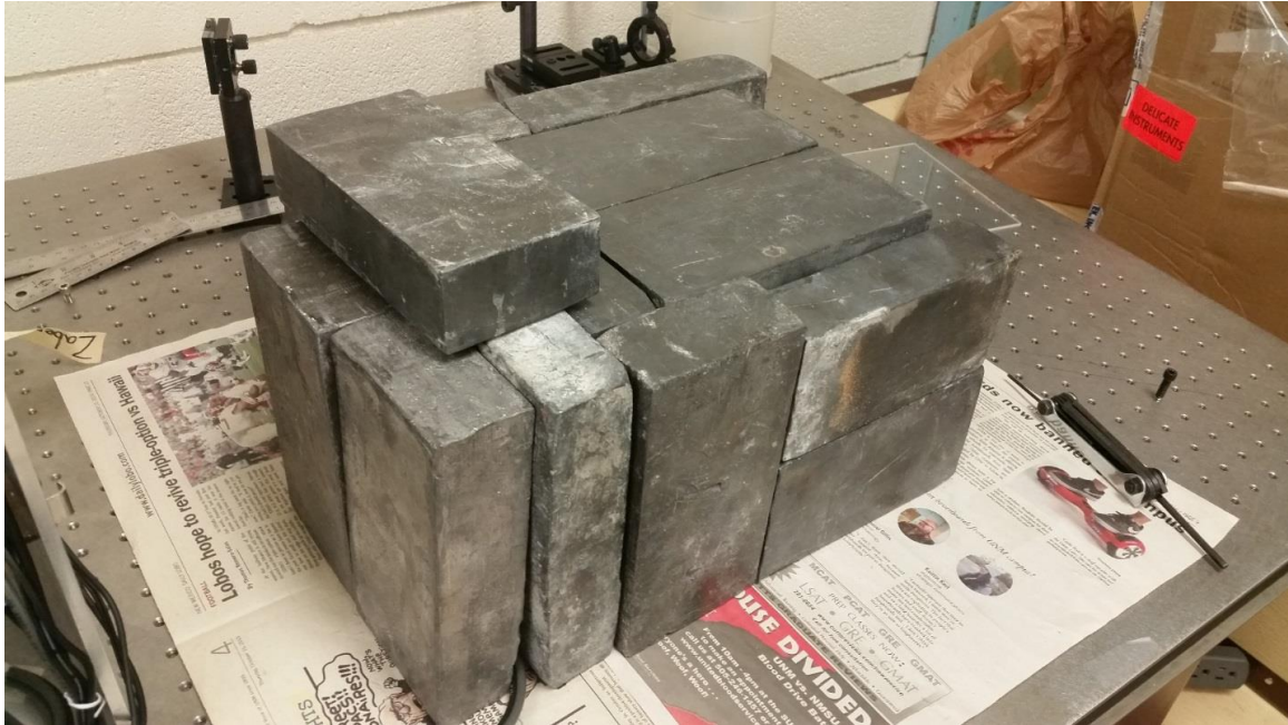
Figure 34: Lead enclosure for detector.
