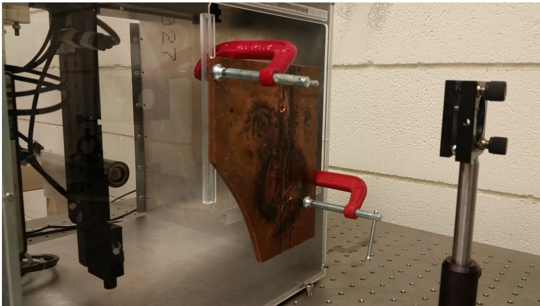
Figure 55: Experimental setup to simulate D-Matrix detector.
